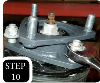
**STEP 11:** Rotate the top hat of the strut 180 using a strut compressor.
