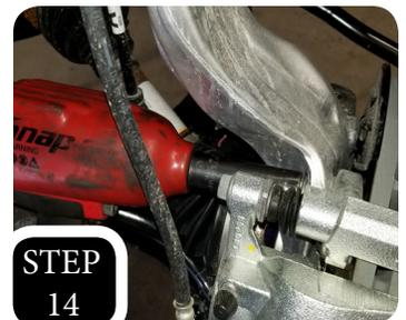
STEP 15: Tighten up the axle using the factory nut.
