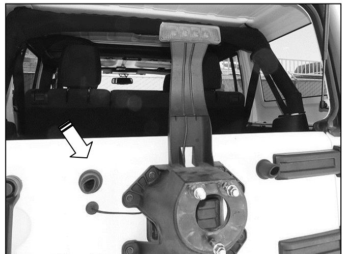
(Fig 2) Release rubber grommet (left arrow) and pull harness through hole in tailgate. Remove plastic spare tire mount from tailgate.
