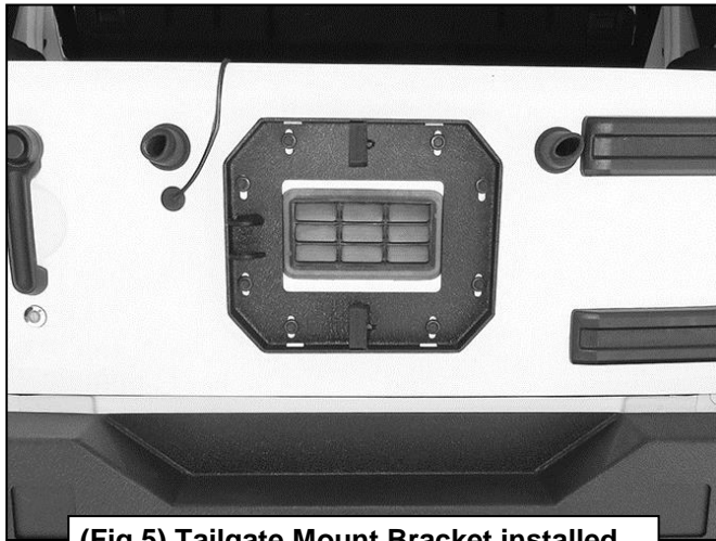
(Fig 5) Tailgate Mount Bracket installed
