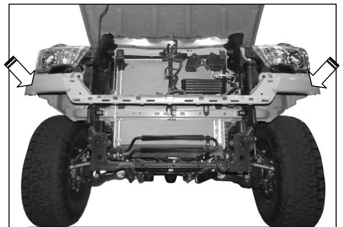
(Fig 16) Use the factory clips and bolts to attach the trimmed Front Bumper (arrows)
