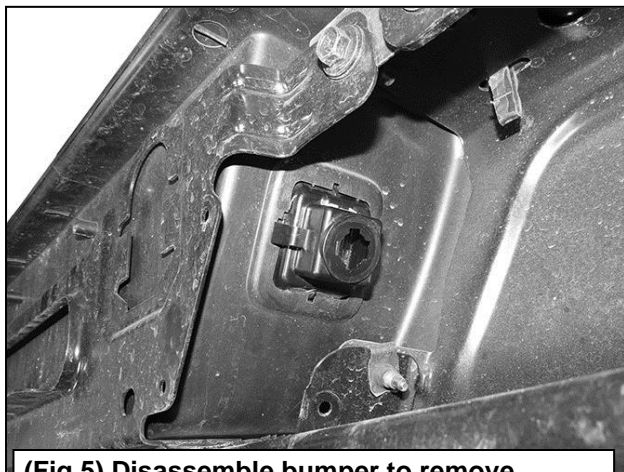
(Fig 5) Disassemble bumper to remove license plate lights, trailer plug, sensors and wiring harness from bumper as equipped
