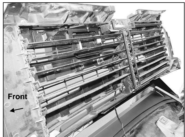
(Fig 19) F-150 Models. Plug harness into sensor. Check fit of harness, secure harness to grille. Rewrap wiring harness. Reinstall shutter blades. Reinstall grille assembly
