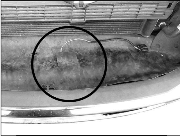
(Fig 16) F-150 Models. On installations using factory bumper, cut an opening in the rubber splash guard approximately 3" back from front edge
