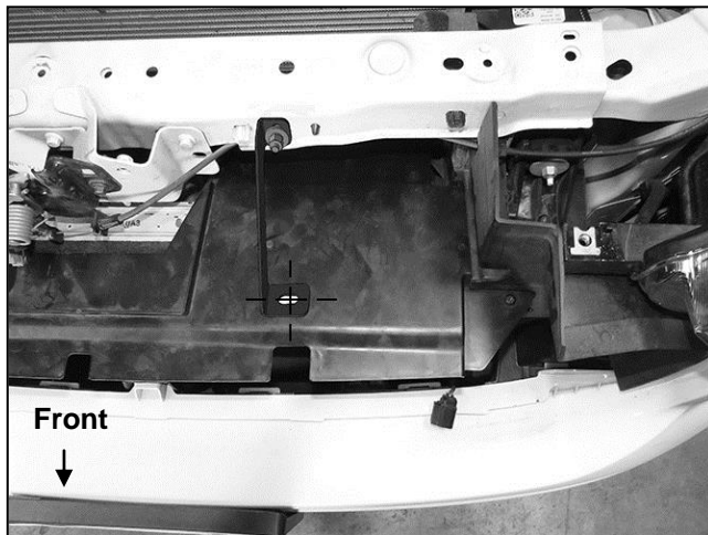
(Fig 26) Ranger Models. Reinstall plastic inner shield. Attach Support Bracket to front of radiator core support. Mark location of slot in Support Bracket onto top of plastic shield. Remove shield and drill a 5/16" hole through marked location. Reinstall shield
