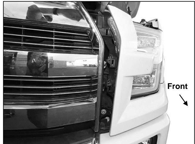
(Fig 3) F-150 Models. Pull out plastic headlight surround to access grille hardware along sides
