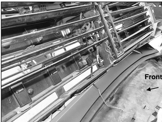
(Fig 18) F-150 Models. Push sensor plug up through opening. Pull harness up between shutter blades and grille to sensor. NOTE: Temporarily remove shutter blades as necessary for access to harness and sensor
