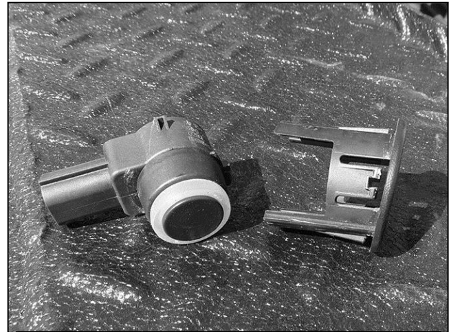
(Fig 9) Remove the sensor from the mount (right) . Remove seal from end of sensor. Push Foam Seal onto end of sensor (Fig 10)
