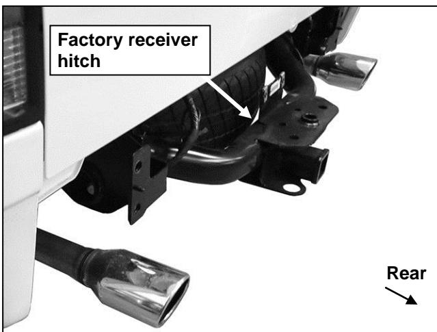
(Fig 5) Bumper completely removed (1500 model pictured)
