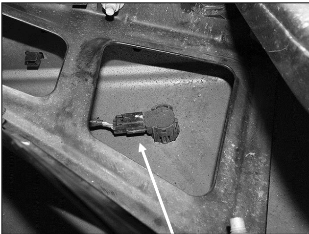
(Fig 8) Unplug the sensor first then remove the sensor from the mount. Disassemble bumper to remove all sensors and harness as equipped
