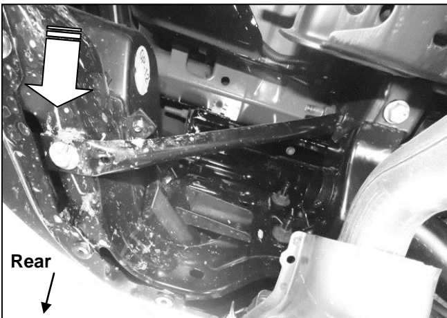
(Fig 5) Remove the bolts attaching the outer bumper supports to the bottom of the bumper (arrow)
