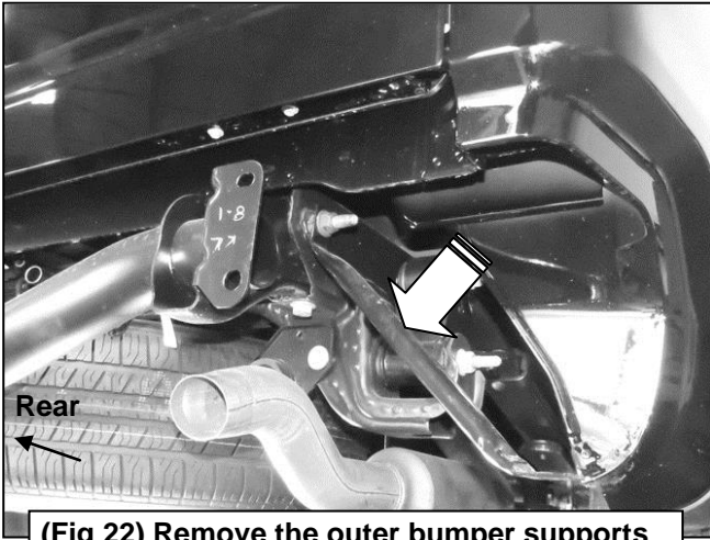
(Fig 22) Remove the outer bumper supports from both sides of the frame (arrow)
