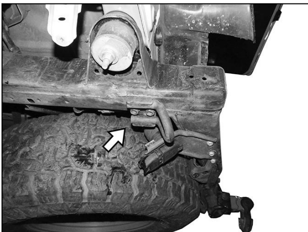
(Fig 16) Remove both tow hooks attached to bottom of frame (arrow-driver/left side pictured)
