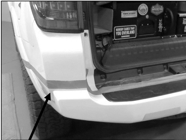
(Fig 12) Cut along guidelines (driver/left corner of bumper cover pictured)
