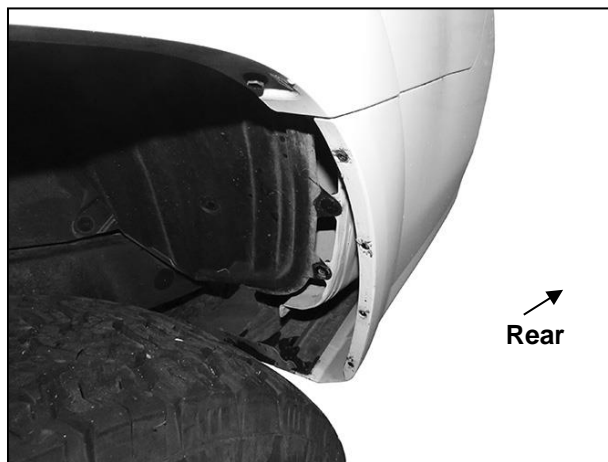
(Fig 4) Plastic cover and mud flap removed
