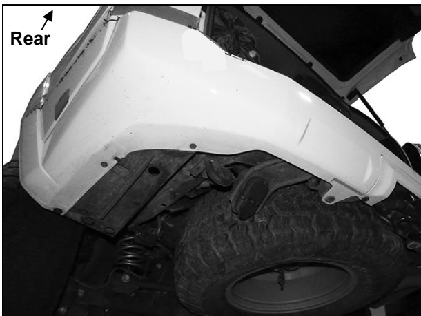
(Fig 14) Remove clips/hardware attaching bottom of bumper cover (driver/left pictured)
