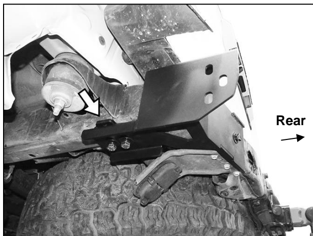
(Fig 23) Insert Shims between frame and Bracket as needed to level/align Bumper to vehicle (see Step 16)
