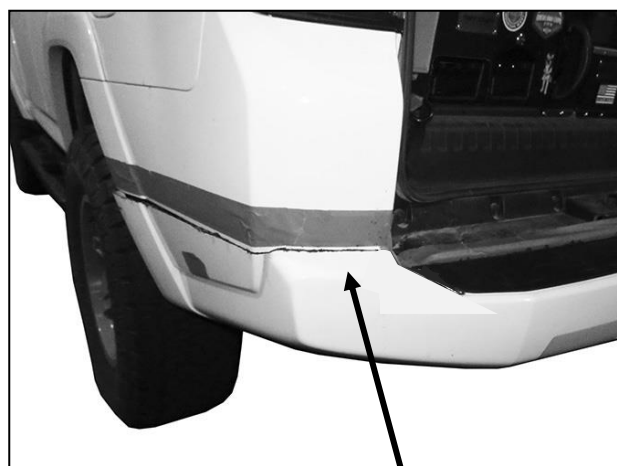
(Fig 11) Cut along guidelines (driver/left corner of bumper cover pictured)
