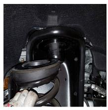
**STEP 8:** Lower the axle enough to remove the coil and the upper rubber coil isolator.
