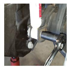
**STEP 3:** Working on one side at a time. Unbolt the shock and separate from the vehicle.
