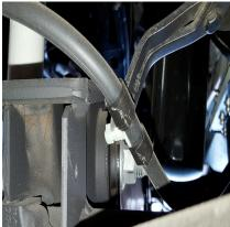
**STEP 5:** Remove the stock brake line bracket from the bottom of the stock coil spring seat. Then, unclip any abs lines or vent lines that may get stretched out when lowering the axle.
