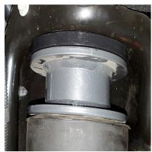
**STEP 9:** Locate the new coil spring spacers & the new isolators. Install the factory isolator on the coil, then the spacer, then the urethane pad: next jack up the axle until coil spacers on top of the driver's side coil spacer seats properly
