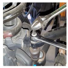
**STEP 4:** Next, unbolt the sway-bar end link on the sway bar side on both driver and passenger sides.
