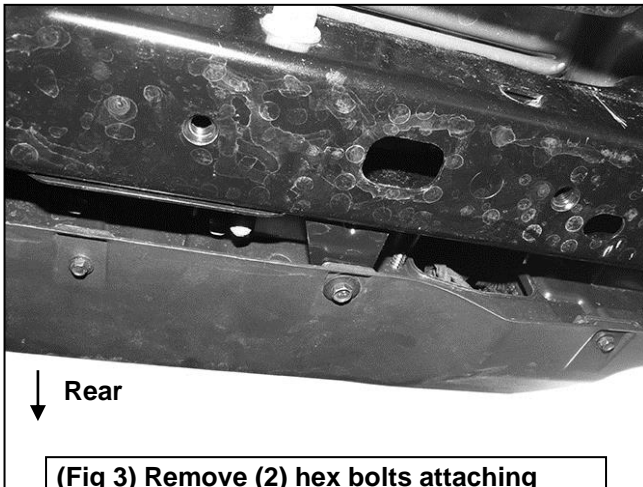
(Fig 3) Remove (2) hex bolts attaching bottom of bumper to frame cross member
