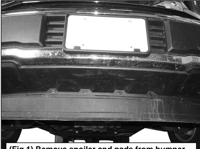
(Fig 1) Remove spoiler and pads from bumper
