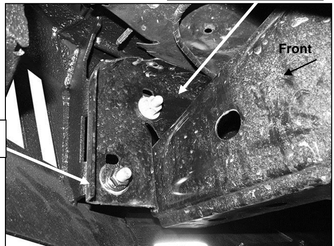
(Fig 8) Reuse factory hardware to attach Bumper to frame mounting flange
