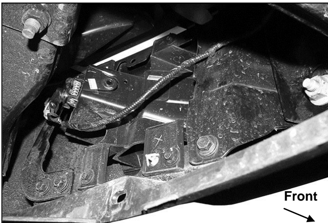
(Fig 3) Unplug and move factory wiring harness for fog lights (if equipped)
