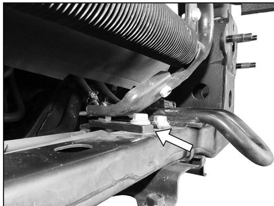
(Fig 19) Passenger/right side of cooler relocated towards the radiator (arrow)
