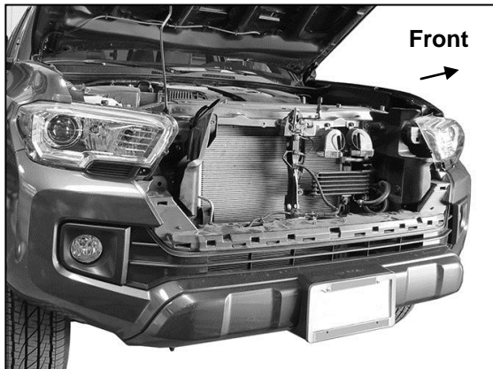
(Fig 11) Grille Removed. Remove factory bumper bolts along the top and bottom of bumper cover
