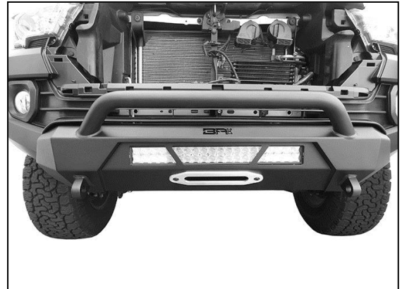
(Fig 33) Check fit of Bumper to plastic and trim as necessary. Reinstall grille and top cover
