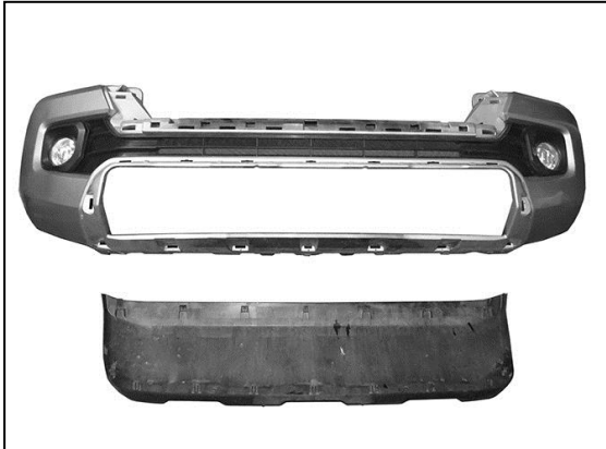
(Fig 22) Remove center pad from bumper cover
