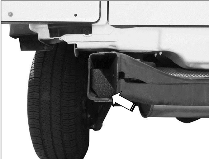
(Fig 5) Insert 14mm Double Nut Plate into open end of frame (driver/left side pictured)
