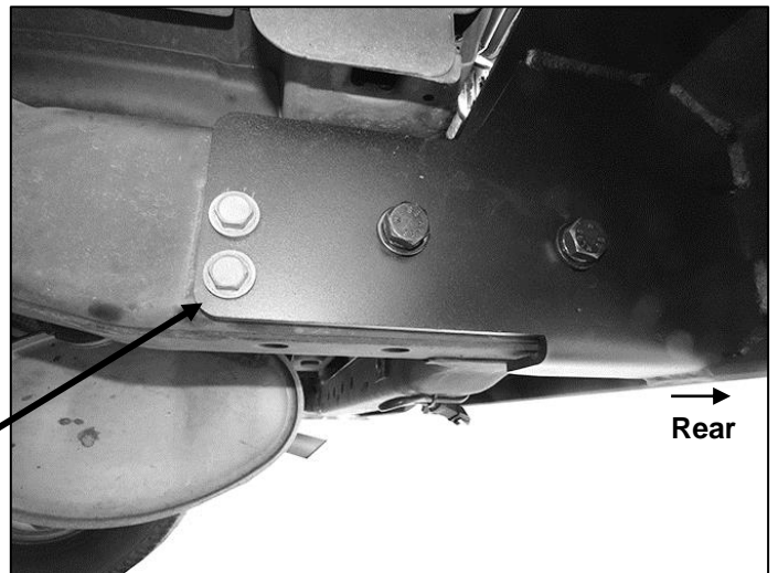
(Fig 8) Attach the driver/left side of the Bumper to the Nut Plate in frame and threaded holes
