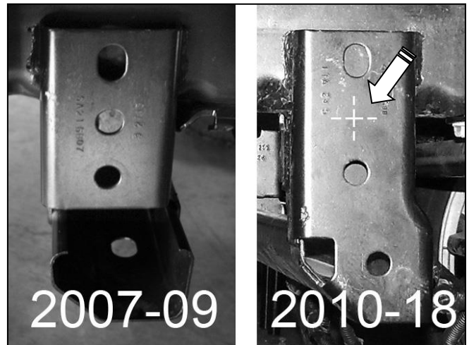
(Fig 6) Determine year of vehicle, 2010-18 models will require drilling 1/2" hole in bracket on outside of frame for support bolts
