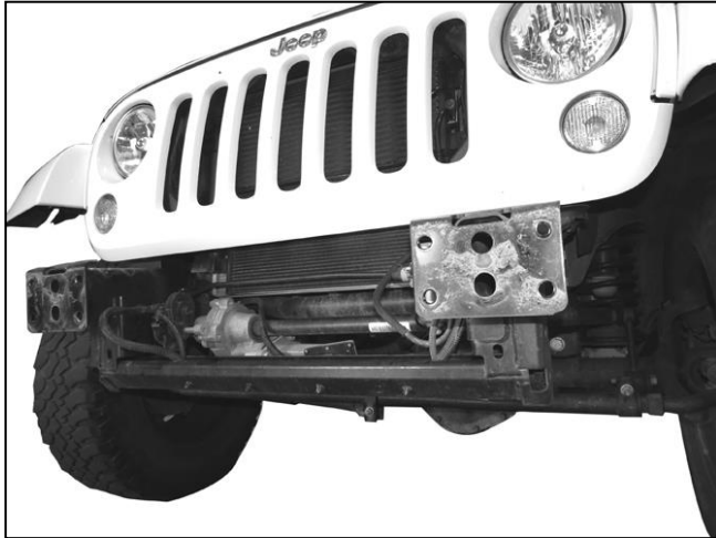
(Fig 3) Front Bumper and splash guard removed. NOTE: Check (8) mounting bolt holes for fit, holes may need to be drilled to 1/2"
