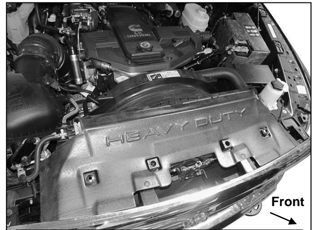
(Fig 2) Open hood and remove plastic cover
