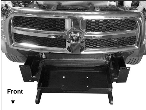
(Fig 10) Attach Winch Tray to Frame Brackets
