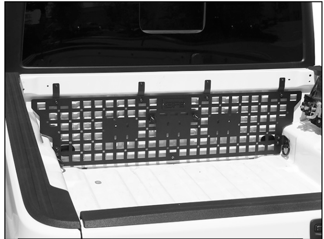
(Fig 14) Complete installation of Panel only
