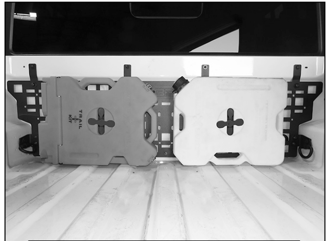
(Fig 8) Example of container installation. Panel features (3) predrilled mounting locations. Attach all desired accessory brackets (not included) to Panel before attaching Panel to Mounting Brackets
