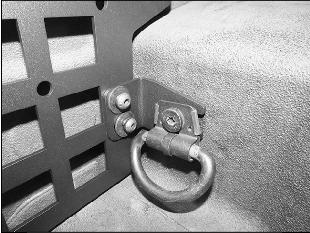
(Fig 13) Reinstall the factory cargo tie down loop over the Lower "L" Bracket
