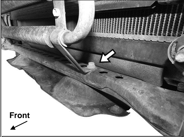
(Fig 11) Remove hex bolt attaching driver/left side of cooler to frame crossmember (arrow)
