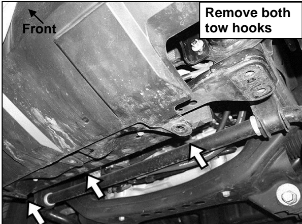
(Fig 6) Remove hardware attaching plastic cover on bottom of bumper to cross member (arrows), Remove tow hooks
