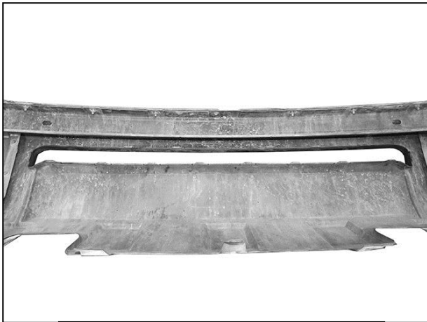
(Fig 17) Remove upper grille from back of plastic bumper section
