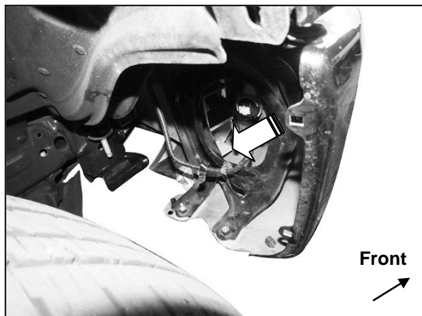
(Fig 5) Disconnect fog lights and move wiring harness away from bumper (arrow). Passenger side of bumper pictured
