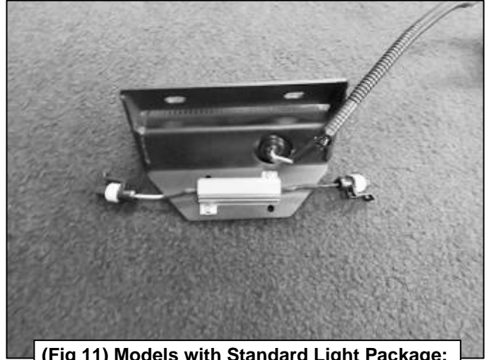
(Fig 11) Models with Standard Light Package: Install resistor on the inside of the turn lights
