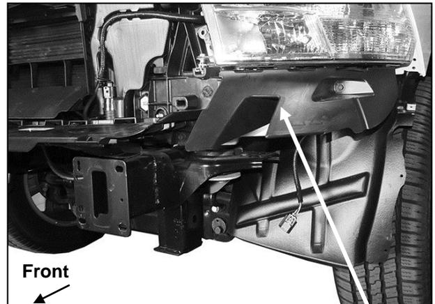
(Fig 6) Remove plastic block from below headlight
