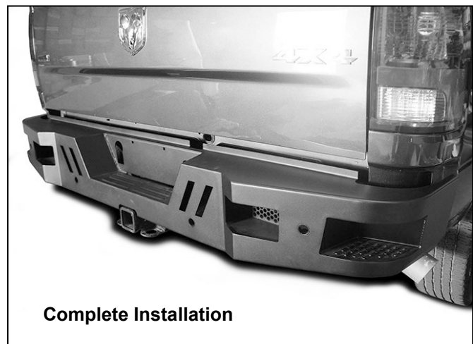
(Fig 13) Push plastic plugs into holes for license plate. Install License Plate Light and trailer plug
