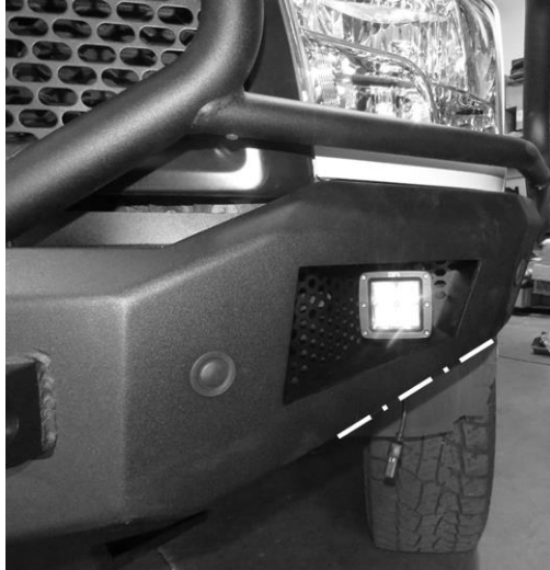
(Fig 17) Trim fender liners as desired using sharp knife or hacksaw
