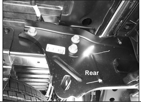
(Fig 2) Models without factory receiver hitch: Remove factory hex bolts attaching bracket to side of frame (driver/left side pictured)
