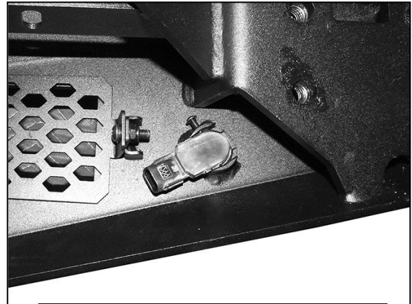
(Fig 13) Use 4mm Screws to lock sensor in place, if necessary, (Fig 11). Plug wiring harness into sensors
