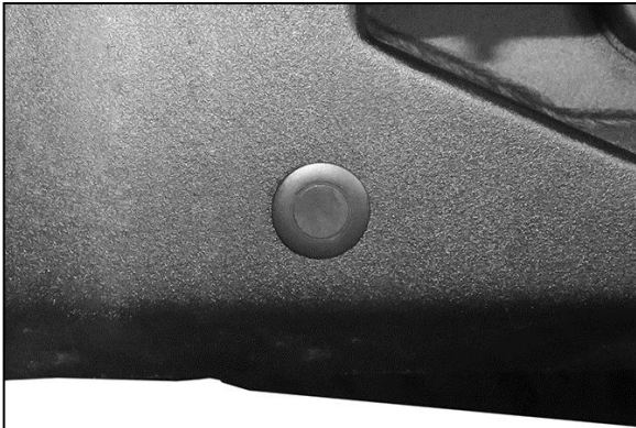
(Fig 12) Push sleeve into sensor mount in Bumper first, then from the back, snap sensor into sleeve (Fig 13)
