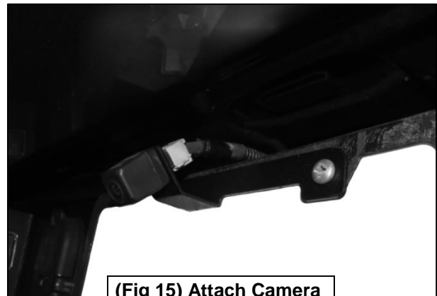
(Fig 15) Attach Camera to notch in Bracket
