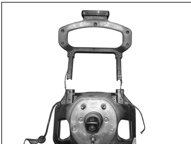
(Fig 21) Remove the light bracket from the top of the factory tire mount
