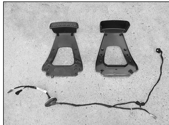
(Fig 19) Disassemble the brake light to unplug and remove the wiring harness
