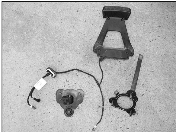
(Fig 22) Models with camera, unplug camera and separate camera from steel bracket
