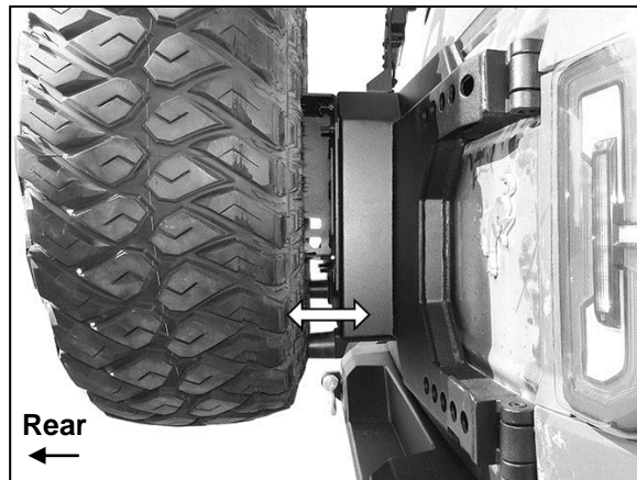
(Fig 34) Adjust rubber bumpers in or out to support the spare tire
