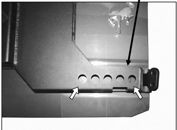
(Fig 11) Insert Hex Bolts into right side of Tire Carrier and into the top and bottom hinge mounting holes in the door (arrows-bottom hinge pictured. Also see Fig 10)
