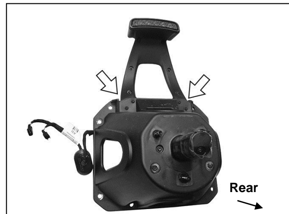
(Fig 17) Remove the brake light assembly from the top of the spare tire mount
