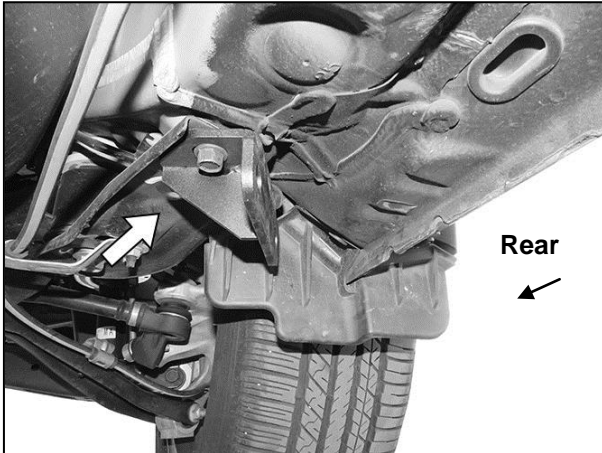
(Fig 6) Driver/left rear Mounting Bracket installed on model with "stock" suspension, no suspension lift spacer.
