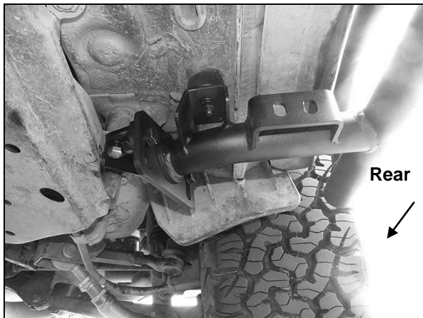
(Fig 18) Models with suspension lift "spacer," attach Adjustable Mounting Plate on end of Rocker Slider to rear Frame Bracket
