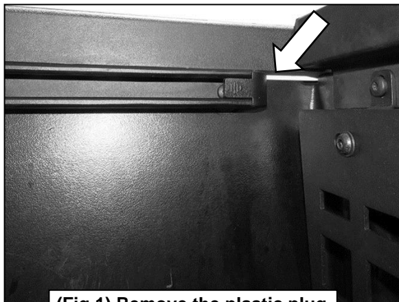
(Fig 1) Remove the plastic plug at the end of the bedrail
