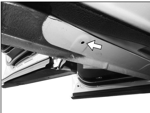
(Fig 10) Use a 3/8" drill bit to enlarge mounting holes in floor for Insert installation (arrow). Do not drill through floor
