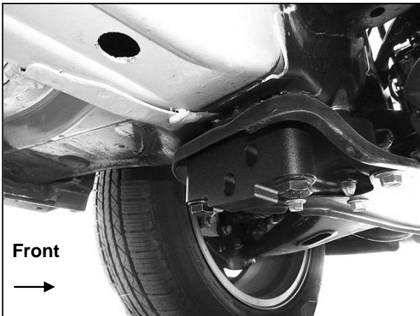
(Fig 5) Driver/left Front Frame Bracket installed
