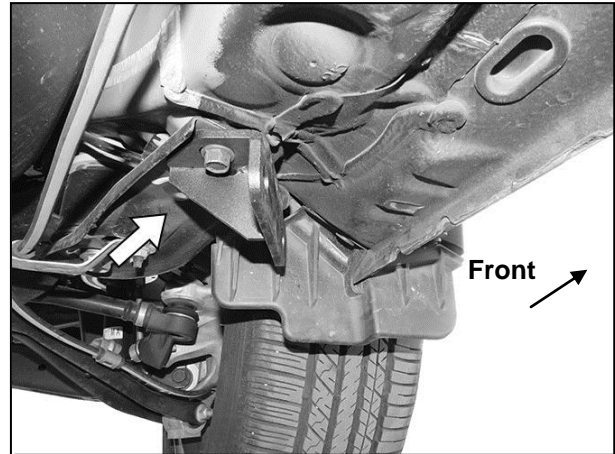
(Fig 17) Models without suspension lift "spacer." Reuse factory hex bolts to attach rear Frame Mounting Bracket (driver/left rear Frame Bracket installation pictured-arrow)
