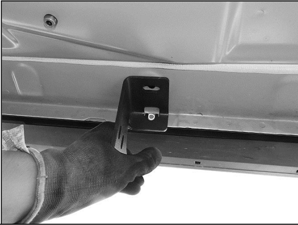
(Fig 7) Hold Bracket up to floor. Line up center of slot with existing hole. Mark location of mounting slot onto back of pinch weld
