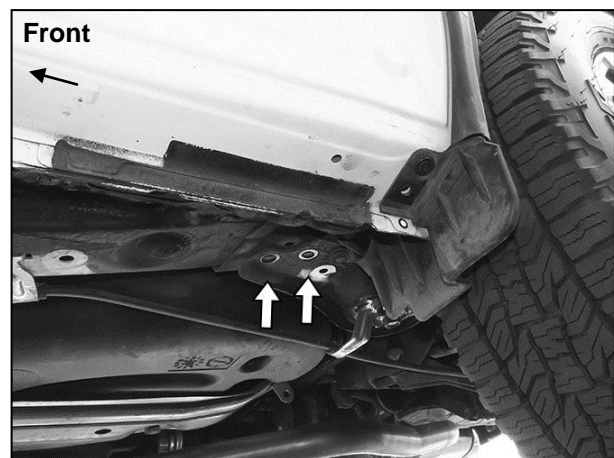
(Fig 15) Remove (2) factory hex bolts (arrows)
