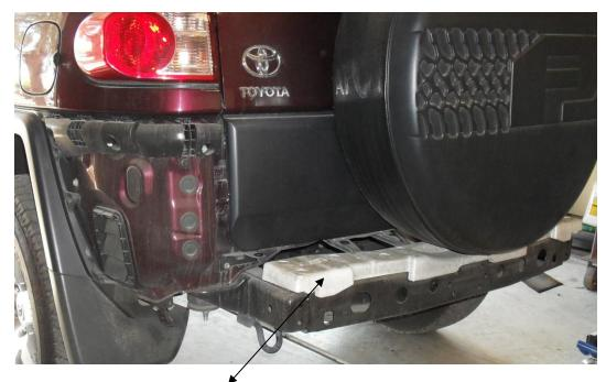
3 Remove Styrofoam center piece.
