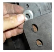
7 Check alignment to body and tighten all hardware. Start with the bolts under the frame, tighten the center bolts last.
