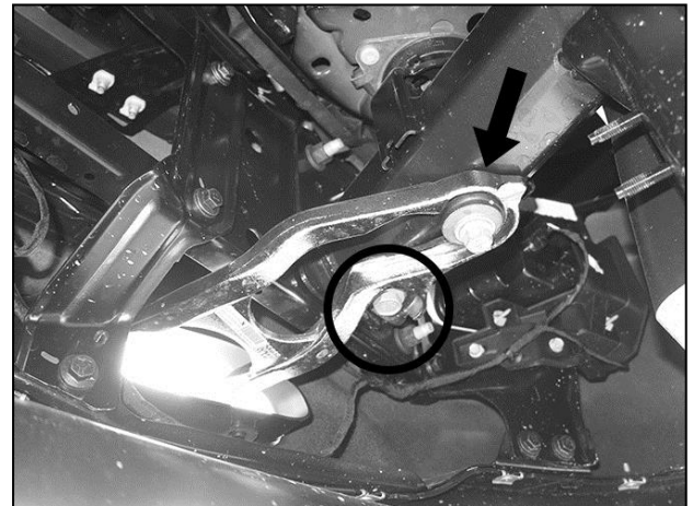
(Fig 4) Loosen but do not remove body bolt (arrow) and remove hex bolt (circle) to remove two hooks (passenger/right side pictured)
