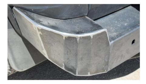
5. Using M12x1.75x40mm bolts, washers and nuts loosely attach D-ring plate to bumper and bumper to vehicle.
