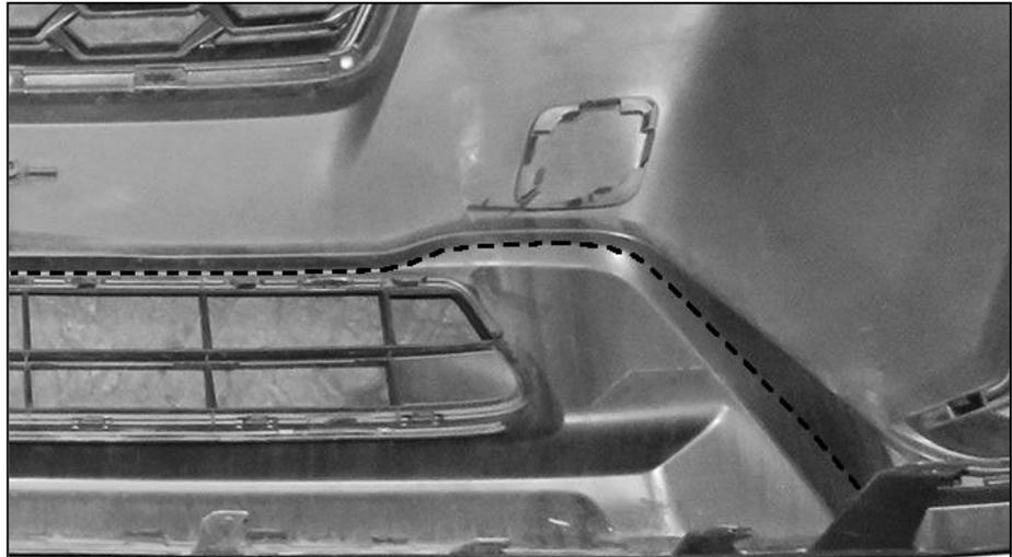
(Fig 21) Use a marker or removable tape to make a cut line along trim line. Dashed line represents suggested final point for cutting, additional trimming may be required for a proper fit. Passenger/right side pictured, draw duplicate line on driver/left side of bumper cover
