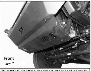
(Fig 21) Skid Plate installed. Note test sample pictured, design may differ
