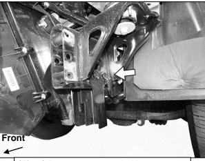
(Fig 2) Bumper removed. Also remove tow hooks and lower frame extensions as equipped (arrow)
