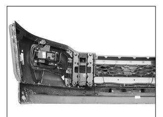
(Fig 8) Remove harness and parking sensors from factory bumper if equipped
