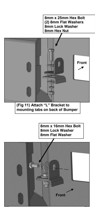
(Fig 13) Attach LED bar style light to "L" Brackets (driver/left side illustrated)
