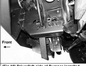
(Fig 19) Driver/left side of Bumper installed
