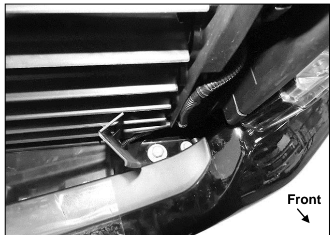
(Fig 6) Pull back cover to locate top bumper bolts
