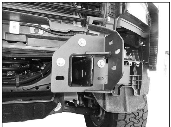
(Fig 10) Driver/left Frame Bracket installed
