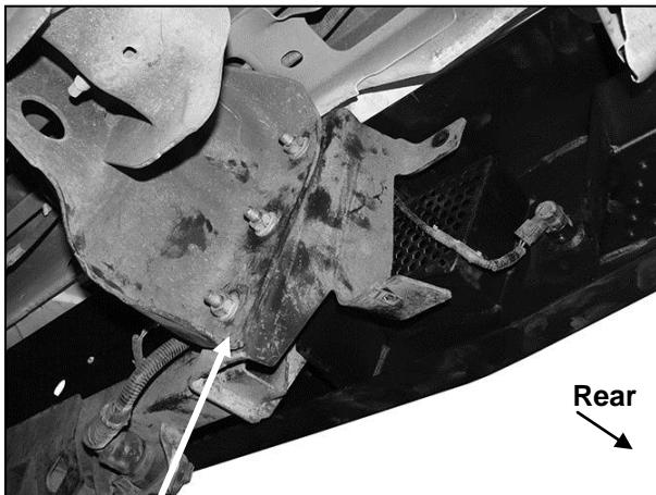
(Fig 11) Reuse factory hex nuts to attach Bumper and receiver hitch to frame
