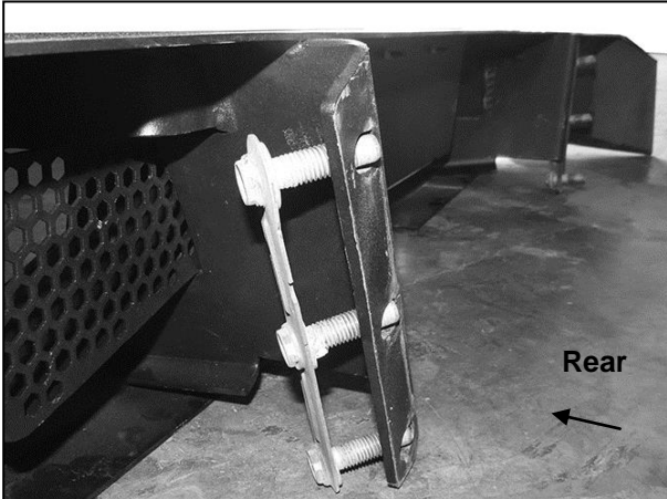
(Fig 9) On models without receiver hitch, reuse triple bolt plate to attach bumper to end of frame
