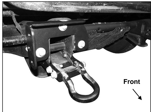
(Fig 9) Attach Tow Hook to Extension Bracket
