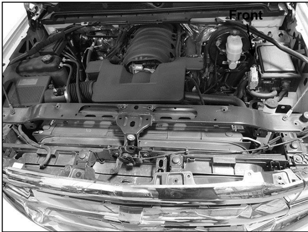
(Fig 1) Remove cover between radiator and grille. Remove screws attaching top of grille
