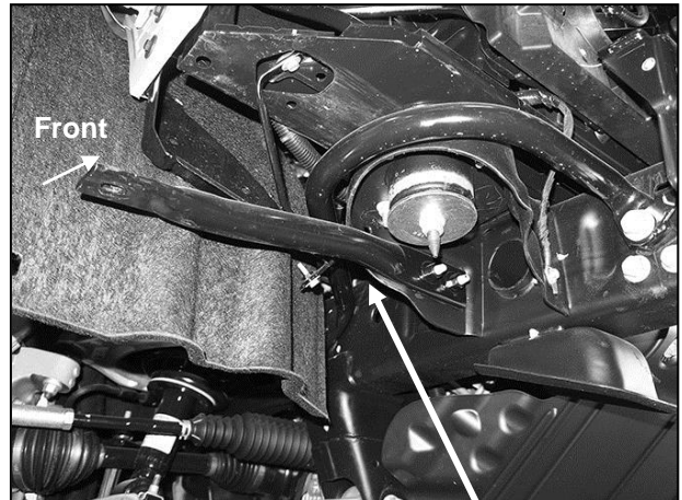
(Fig 4) Remove outer bumper support brackets
