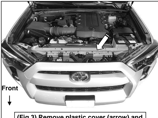
(Fig 3) Remove plastic cover (arrow) and hardware attaching top of bumper cover
