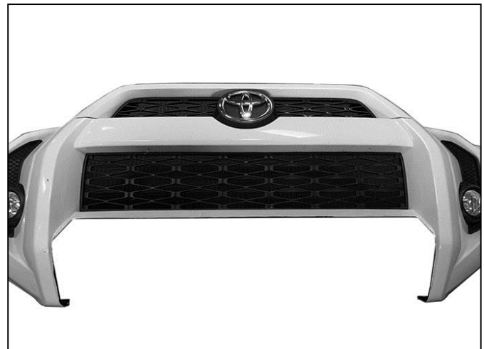
(Fig 14) Clean up cut along plastic and reinstall bumper cover
