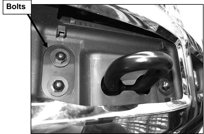
(Fig 6) Remove bumper bolts (driver side pictured)
