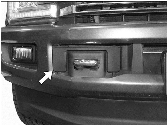
(Fig 3) Remove plastic cover surrounding tow hook (passenger/right side pictured-arrow)
