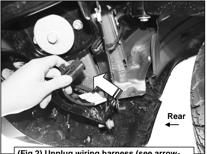
(Fig 2) Unplug wiring harness (see arrow-driver/left side pictured from below bumper)
