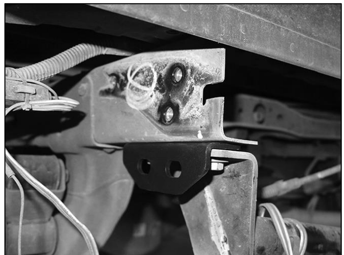
(Fig 7) Attach Support Brackets to bottom of frame. On models without factory hitch or with light duty aftermarket hitch, insert Bracket between bottom of frame and hitch
