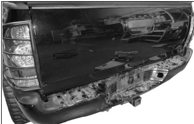
(Fig 3) Models with factory receiver hitch only, remove plastic cover from top of bumper to access hex bolt attaching bumper to top of receiver hitch
