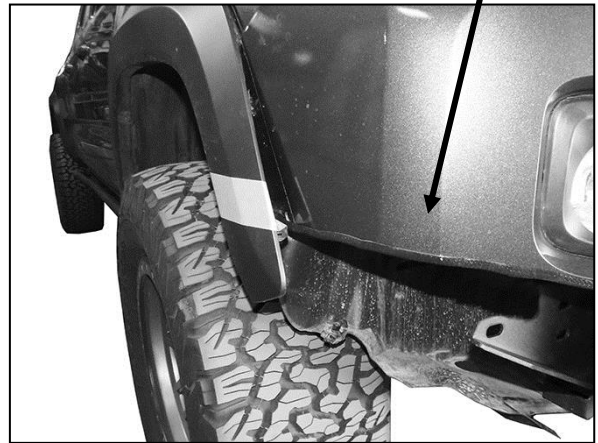
(Fig 18) Use removable tape to protect finish on flare. Cut flare to line up with Wing
