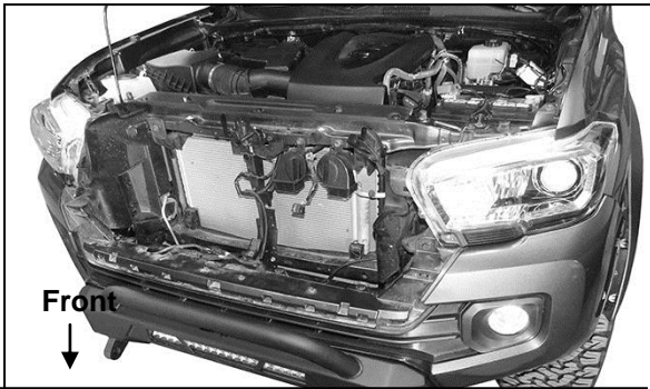
(Fig 3) Cover the top of the bumper with removable tape (masking tape for example)
