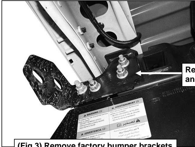
(Fig 3) Remove factory bumper brackets
