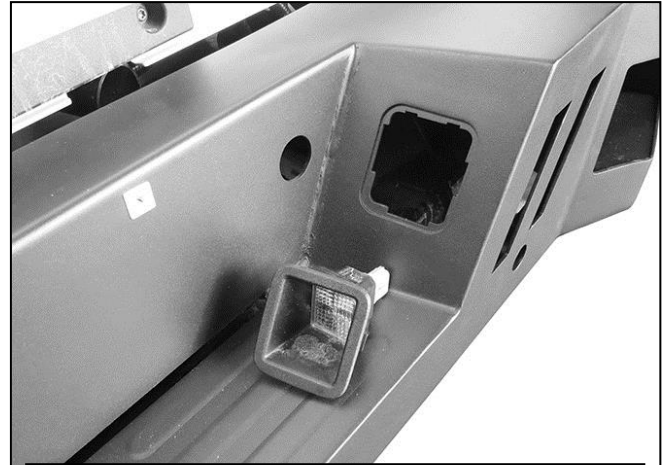
(Fig 9) Push license plate lights into openings
