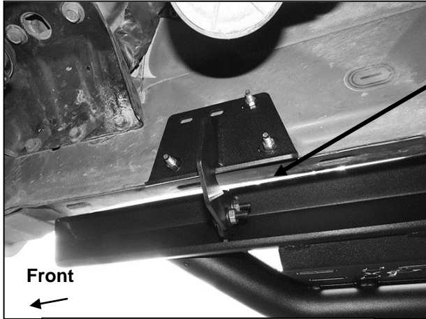
(Fig 9) Passenger/right Side Step attached to front Mounting Bracket
