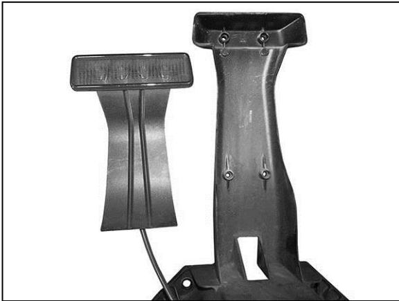
(Fig 18) Remove brake light and harness from top of factory spare tire mount
