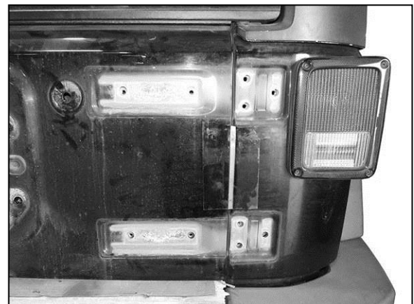
(Fig 4) Remove hex bolts attaching hinges to door. Note scrap wood used along bottom to hold door up in position
