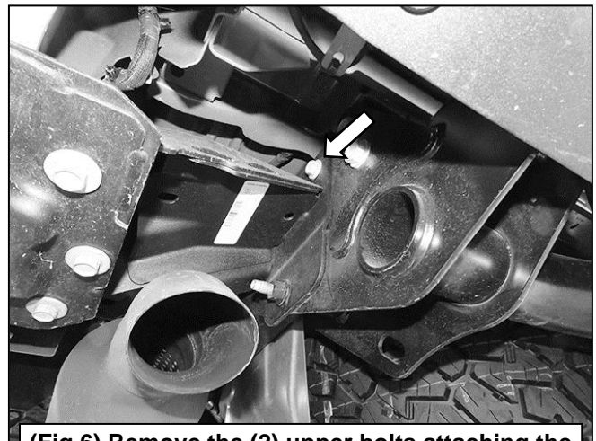
(Fig 6) Remove the (2) upper bolts attaching the bed guard (if equipped) to the receiver hitch
