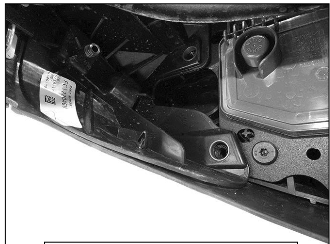
(Fig 2) Steel support bracket removed (Passenger/Right side shown)
