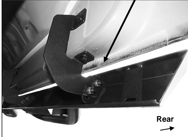
(Fig 15) Attach the passenger/right Side Step to the Mounting Brackets, (rear Bracket pictured)
