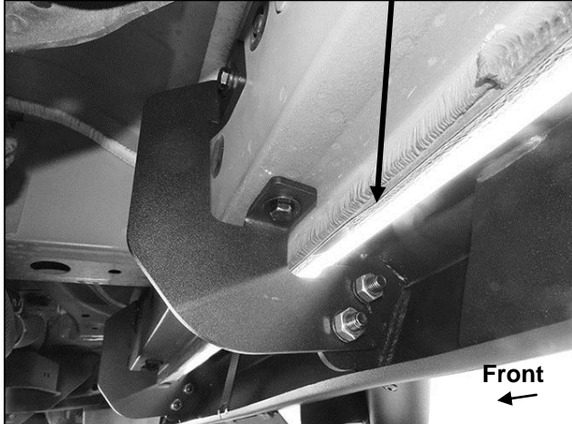
(Fig 14) Attach the passenger/right Side Step to the Mounting Brackets, (#2 Bracket pictured)
