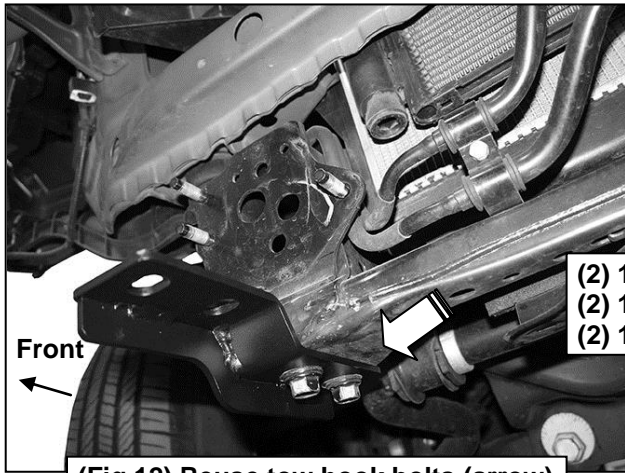
(Fig 12) Reuse tow hook bolts (arrow) to attach passenger/right Support Bracket to bottom of frame
