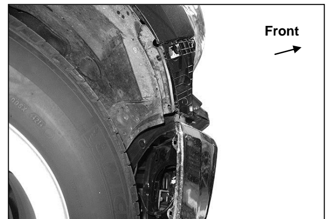
(Fig 6) Plastic cover and fascia body panel removed
