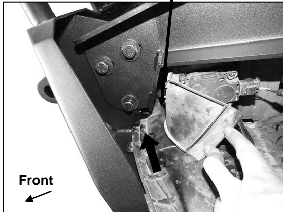
(Fig 17) Insert 12mm "L" Nut Plate into and up behind Bumper (arrow)
