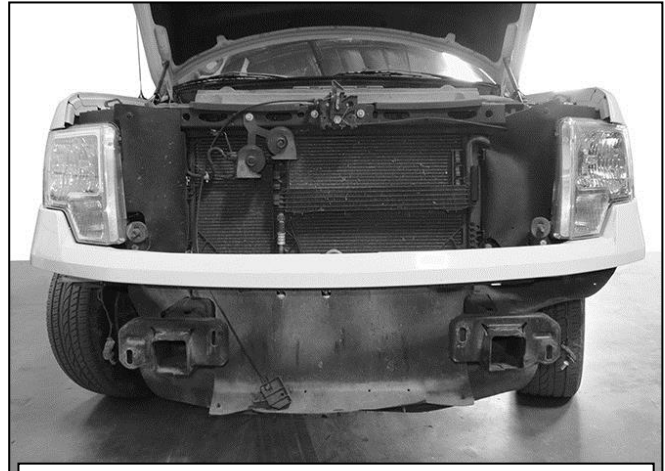
(Fig 6) Remove bumper assembly. Also remove tow hooks and double nut plates if equipped
