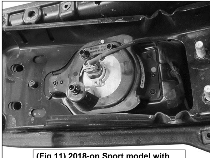
(Fig 11) 2018-on Sport model with 1pc plastic bumper cover. Driver/left Fog light assembly pictured
